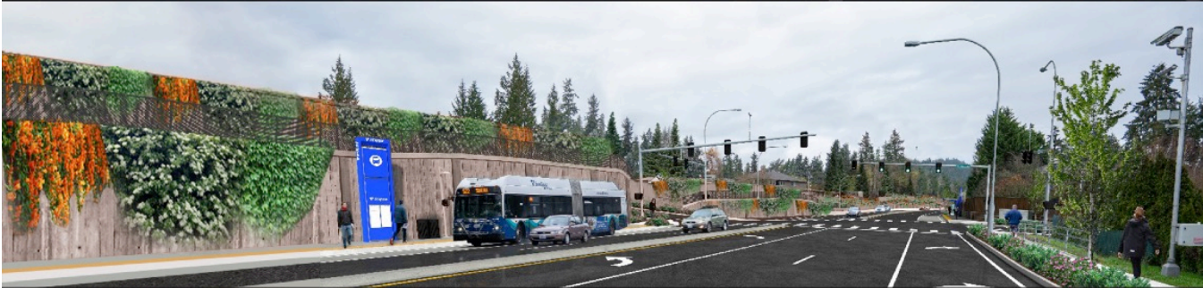
Planted Retaining Walls and Sound Walls with Vines Growing from Top and Bottom
